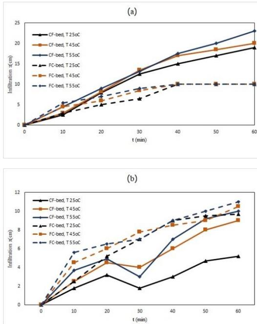
**Fig. 8** Comparison of infiltration front in CF-bed and FC-bed at different supplied water temperatures:
