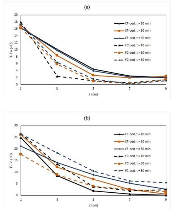
**Fig. 5** Comparison of temperature increase in CF-Bed and FC-Bed at the supplied water flux  $f = 0.15 \text{ kg/m}^2\text{s}$ :
