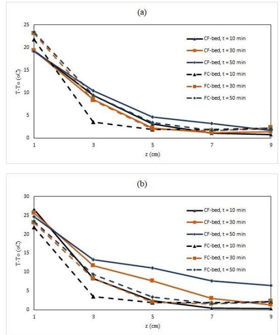
**Fig. 9** Comparison of temperature increase in CF-Bed and FC-Bed at the supplied water flux  $f = 0.20 \text{ kg/m}^2\text{s}$ :
