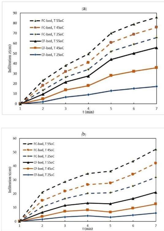
**Fig. 4** Comparison of infiltration front in CF-bed and FC-bed at different supplied water temperatures:
