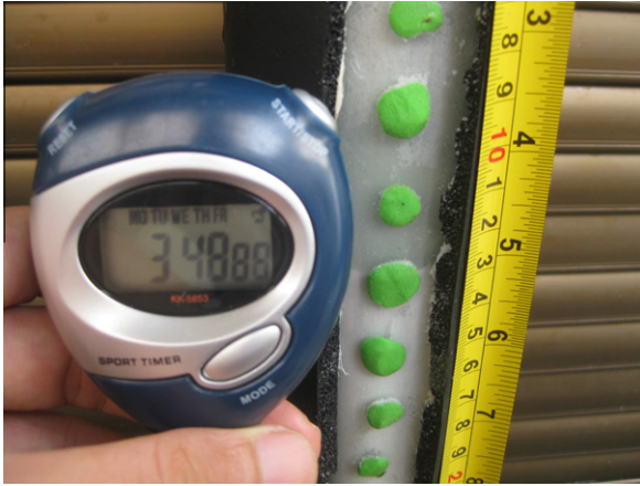
Fig. 2. Experimental apparatus for measuring infiltration depth of water.
