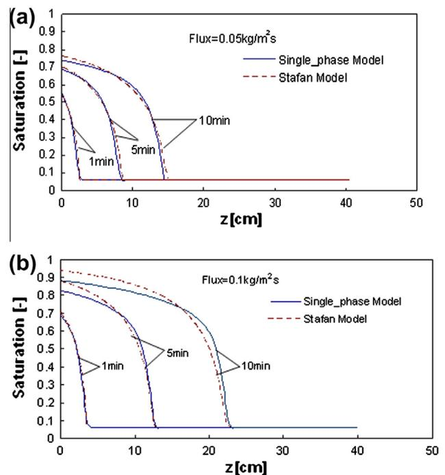
Fig. 5. Comparison of infiltration layer along granular packed bed ( $d = 0.15$  mm) between two models at various elapsed times as a parameter of supplied water flux: (a)  $f = 0.05$  kg/m<sup>2</sup> s and (b) 0.1 kg/m<sup>2</sup> s.
