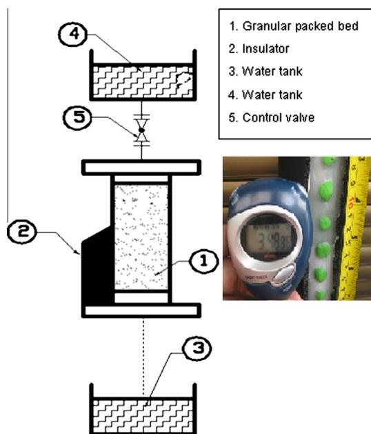
Fig. 4. Experimental apparatus for measuring unsaturated flow in one dimension porous layered.
