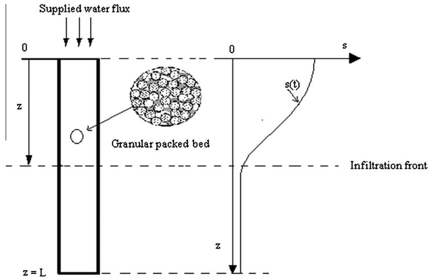
Fig. 1. Schematic representation of the water infiltration in porous media described by the Single-phase model.
