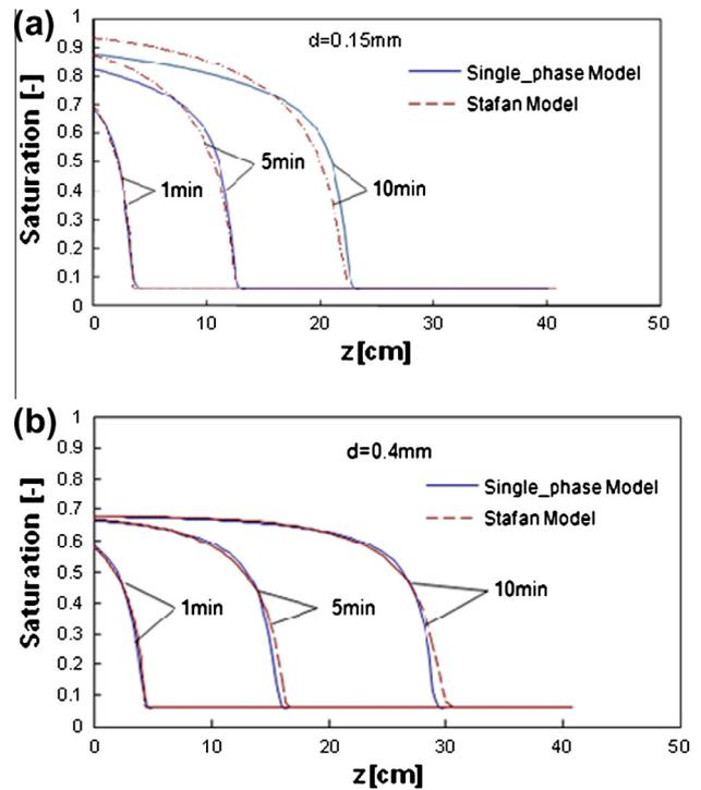
Fig. 7. Comparison of infiltration layer along granular packed bed ( $f = 0.1$  kg/m<sup>2</sup> s) between two models at various elapsed times as a parameter of particle sizes: (a)  $d = 0.15$  mm and (b)  $0.4$  mm.
