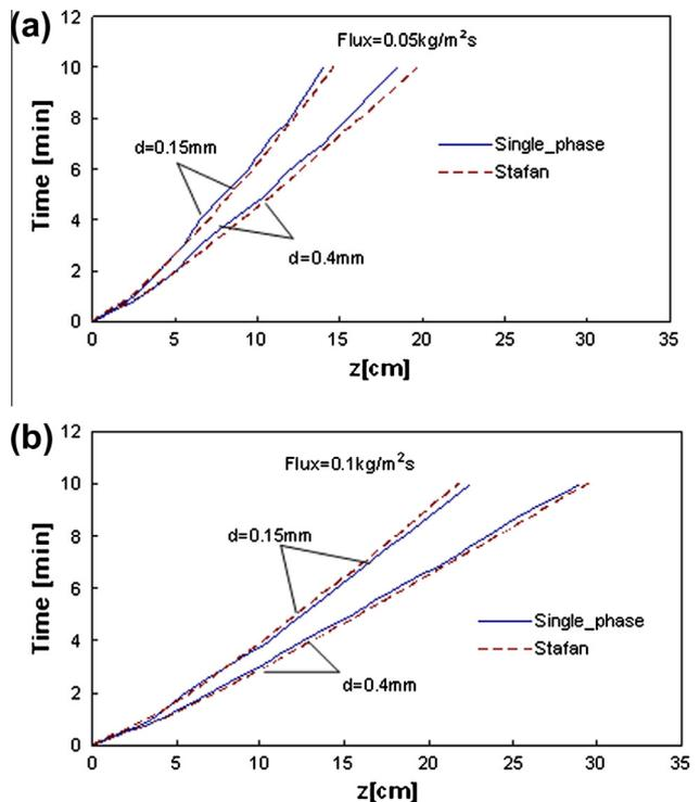
Fig. 8. Comparison of infiltration front ( $d = 0.15$  mm and  $d = 0.4$  mm) between two models as a parameter of supplied water flux: (a)  $f = 0.05$  kg/m<sup>2</sup> s and (b)  $0.1$  kg/m<sup>2</sup> s.
