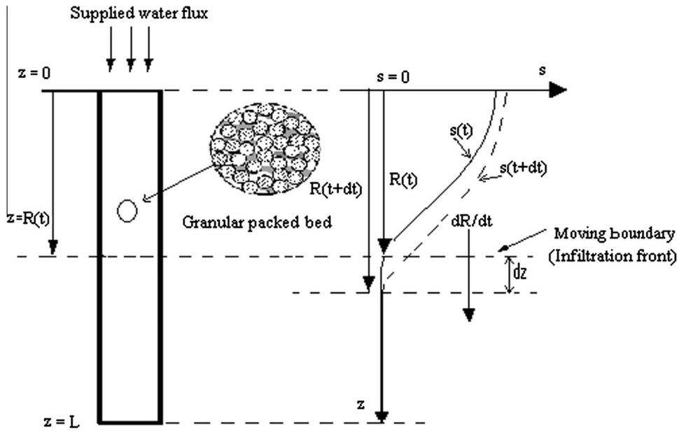
Fig. 3. Schematic representation of the water infiltration in porous media described by the Stefan model.
