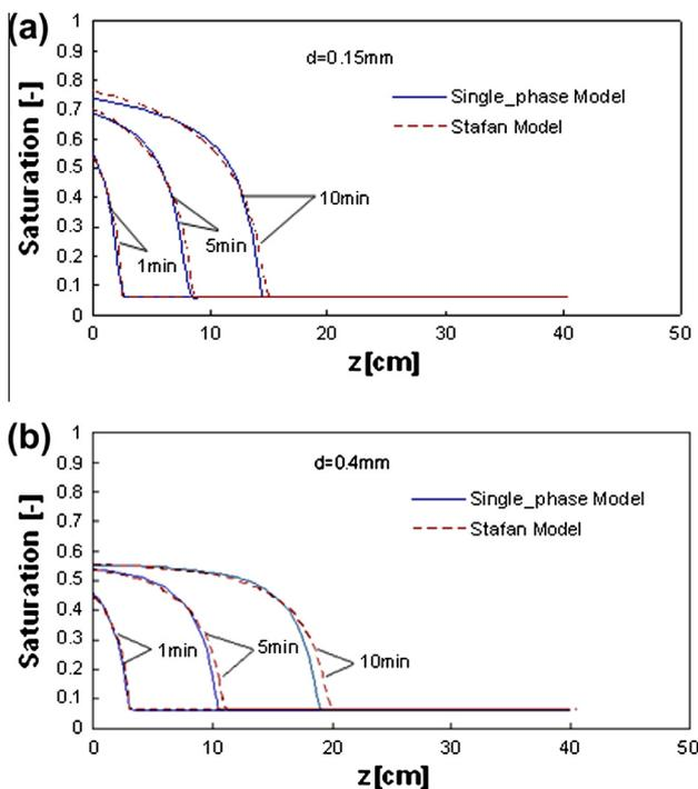
Fig. 6. Comparison of infiltration layer along granular packed bed ( $f = 0.05$  kg/m<sup>2</sup> s) between two models at various elapsed times as a parameter of particle sizes: (a)  $d = 0.15$  mm and (b)  $0.4$  mm.
