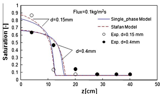
Fig. 9. Comparison of infiltration layer along granular packed bed with different particle size between numerical results and experimental result ( $t = 5$  min,  $f = 0.1$  kg/m<sup>2</sup> s).
