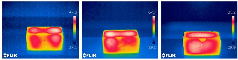
(a) Distribution of surface temperature of CM at a pressure of 30 kPa, w/c of 0.38, magnetron 1, and 12 CM at (a.1) 10 min, (a.2) 40 min, (a.3) 80 min.
