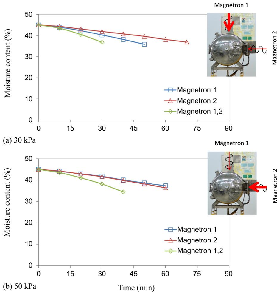
**Fig. 12.** Moisture content and time with a w/c of 0.45 and a pressure of 50 kPa, magnetron positions 1 (vertical magnetron), 2 (horizontal magnetron), and both 1 and 2 for 12 CM specimens.
