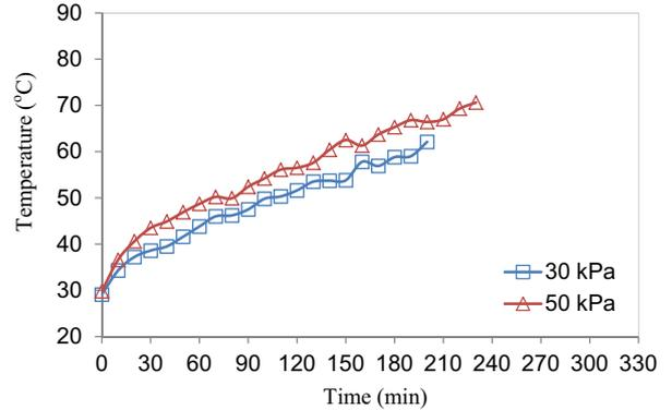
(a) 24 CM specimens, w/c of 0.38, pressures of 30 and 50 kPa, magnetron position 1 (vertical magnetron)
