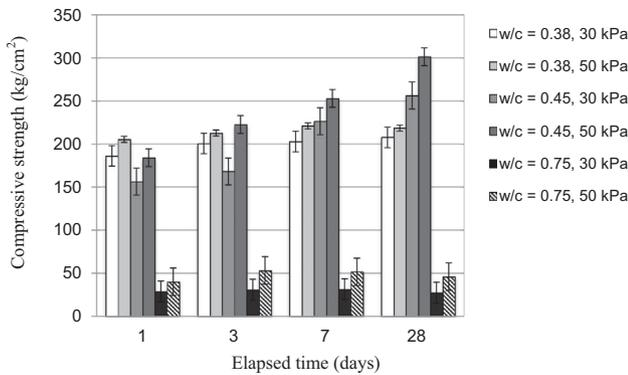
**Fig. 17.** Compressive strengths and elapsed time of CM with w/c values of 0.38, 0.45 and 0.75 at pressure levels of 30 and 50 kPa, magnetron position 1 and 12 CM specimens.
