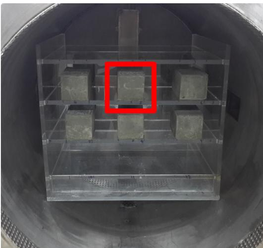
**Fig. 13.** Position used to measure the distribution of the surface temperature of CM.
