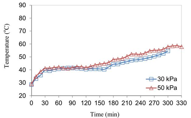
(c) 24 CM specimens, w/c of 0.75, pressures of 30 and 50 kPa, magnetron position 1 (vertical magnetron)
