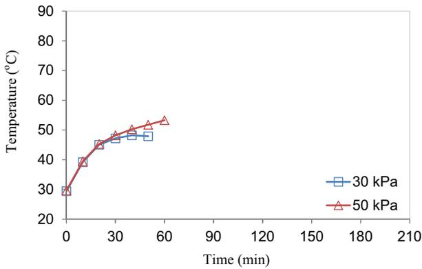
(b) 12 CM specimens, w/c of 0.45, pressures of 30 and 50 kPa, magnetron position 1 (vertical magnetron)
