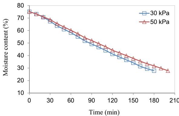
(c) 12 CM specimens, w/c of 0.75, pressures of 30 and 50 kPa, magnetron position 1 (vertical magnetron)
