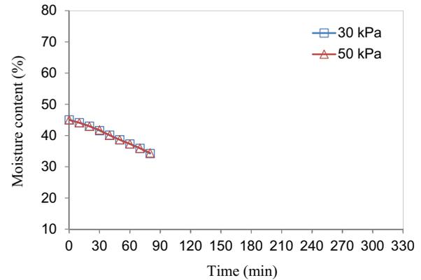
(b) 24 CM specimens, w/c of 0.45, pressures of 30 and 50 kPa, magnetron position 1 (vertical magnetron)
