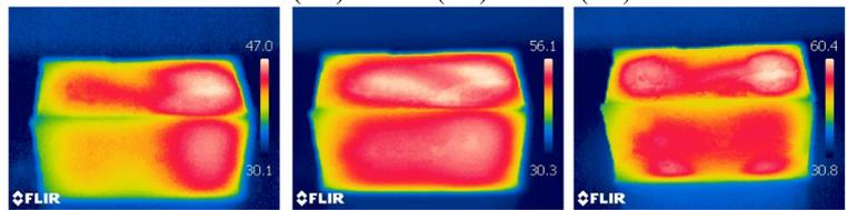
(c) Distribution of surface temperature of CM at a pressure of 30 kPa, a w/c of 0.45, magnetron 1, and 12 CM at (c.1) 10 min (b.2) 30 min (c.3) 40 min
