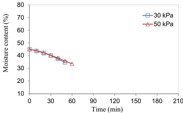
(b) 12 CM specimens, w/c of 0.45, pressures of 30 and 50 kPa, magnetron position 1 (vertical magnetron)
