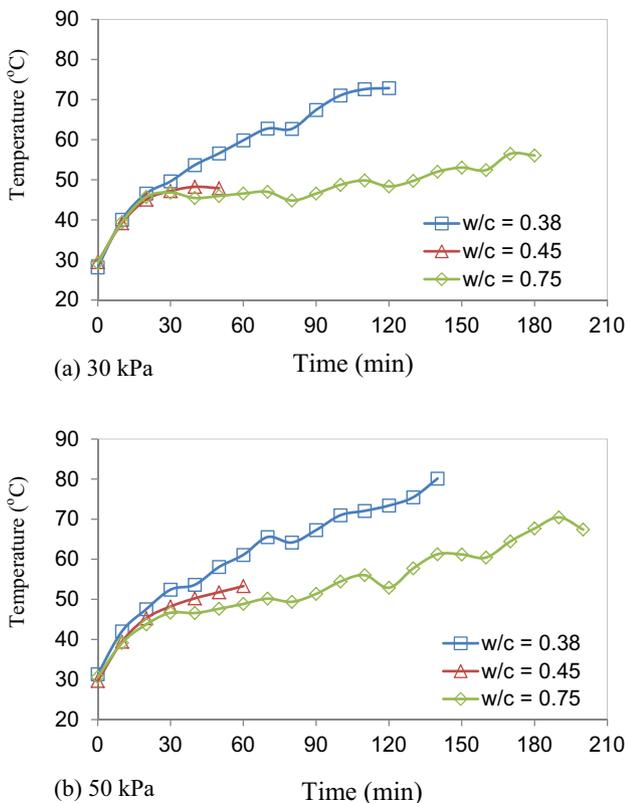
Fig. 7. Temperature and time with w/c values of 0.38, 0.45 and 0.75, magnetron 1 (vertical magnetron), and 12 CM specimens at pressures of (a) 30 kPa and (b) 50 kPa.
