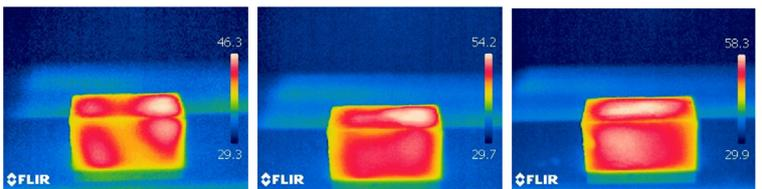
(e) Distribution of surface temperature at a pressure of 30 kPa, a w/c of 0.75, magnetron 1, and 12 number at (e.1) 10 min, (e.2) 40 min, (e.3) 80 min.
