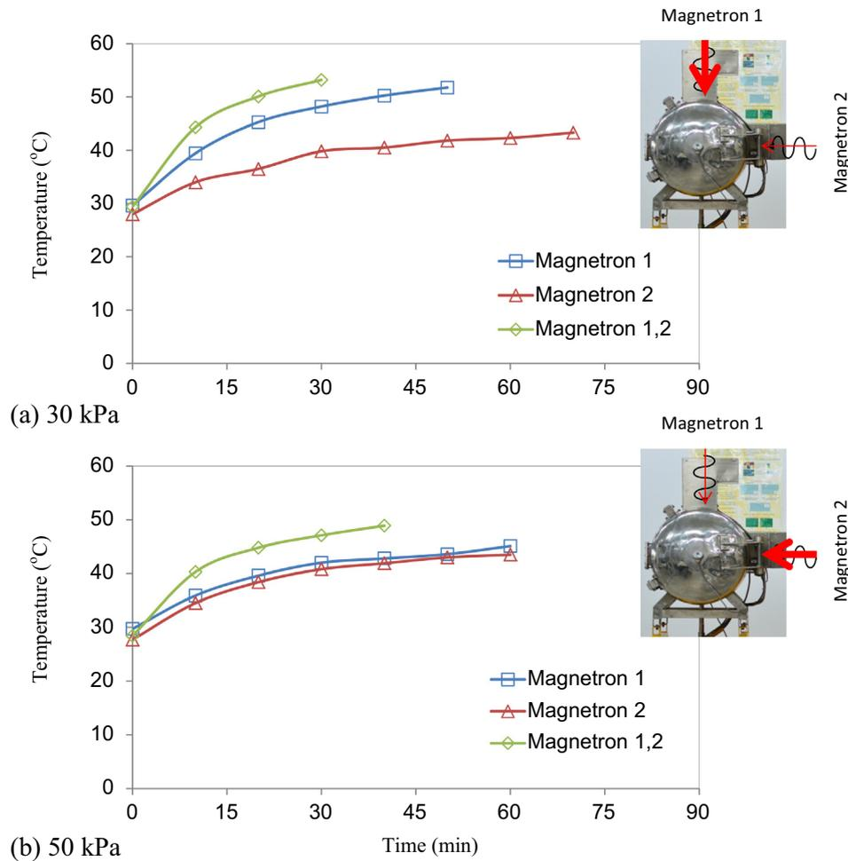
**Fig. 11.** Temperature and time with a w/c of 0.45 and a pressure of 50 kPa at magnetron positions 1 (vertical magnetron) 2 (horizontal magnetron), and both 1 and 2 for 12 CM specimens.
