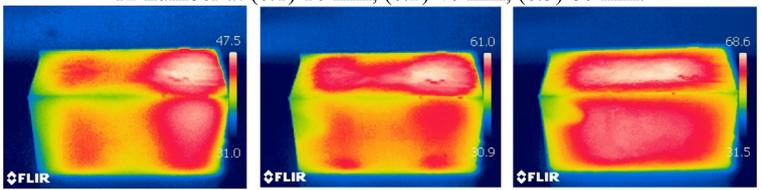
(f) Distribution of surface temperature at a pressure of 30 kPa, a w/c of 0.75, magnetron 1, and 12 CM at (f.1) 10 min, (f.2) 40 min, (f.3) 80 min.
