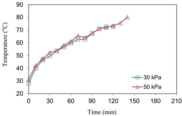
(a) 12 CM specimens, w/c of 0.38, pressures of 30 and 50 kPa, magnetron position 1 (vertical magnetron)
