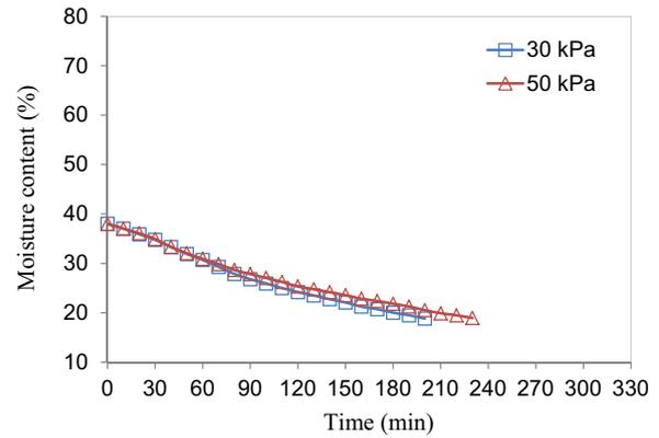
(a) 24 CM specimens, w/c of 0.38, pressures of 30 and 50 kPa, magnetron position 1 (vertical magnetron)
