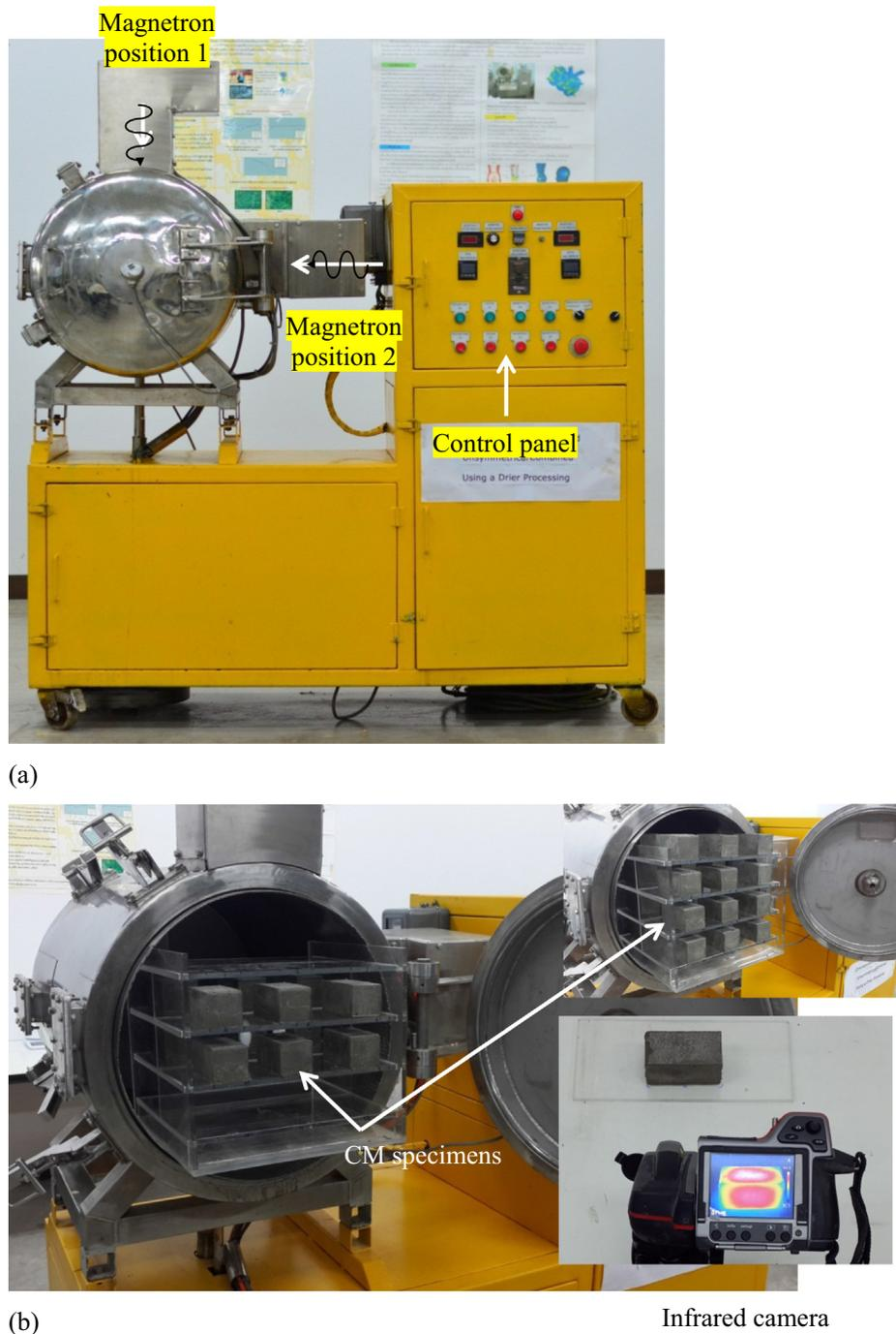
Fig. 2. (a) Commercialized combined unsymmetrical double-feed microwave and vacuum system [22] and (b) CM specimens in MD experiments.
