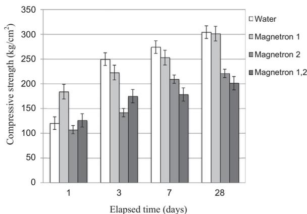
**Fig. 18.** Compressive strength and curing time of CM with the microwave at position 1 (vertical magnetron), magnetron position 2 (horizontal magnetron), and 1 and 2 magnetrons with a w/c of 0.45, a pressure of 50 kPa and 12 CM specimens.
