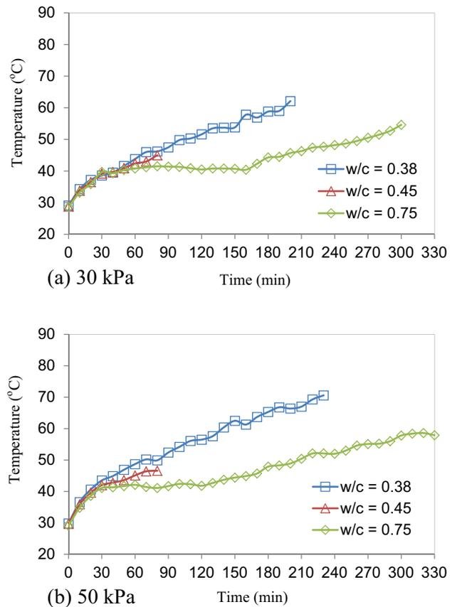
Fig. 8. Temperature and time with w/c values of 0.38, 0.45 and 0.75, magnetron 1 (vertical magnetron), and 24 CM specimens at pressures of (a) 30 kPa and (b) 50 kPa.
