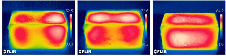
(b) Distribution of surface temperature of CM at a pressure of 50 kPa, w/c of 0.38, magnetron 1, and 12 CM at (b.1) 10 min (b.2) 40 min (b.3) 80 min
