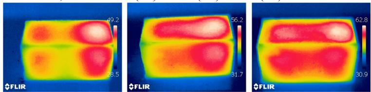
(d) Distribution of surface temperature of CM at a pressure of 50 kPa, a w/c of 0.45, magnetron 1, and 12 CM at (d.1) 10 min (d.2) 30 min (d.3) 40 min
