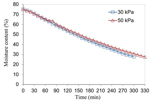
(c) 24 CM specimens, w/c of 0.75, pressures of 30 and 50 kPa, magnetron position 1 (vertical magnetron)
