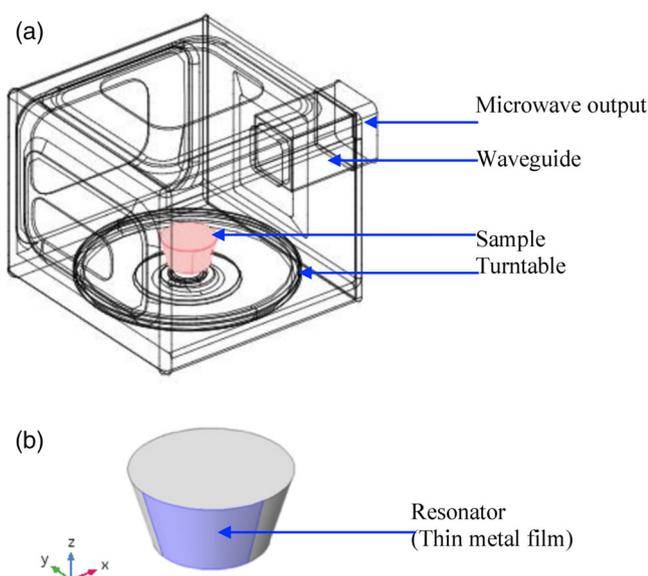
**FIGURE 3** Geometrics of (a) domestic microwave oven and (b) frozen food with resonator
