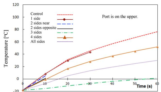
FIGURE 8 The average calculated temperature inside the sample during microwave heating for 60 s at various resonator areas: case of upper port
