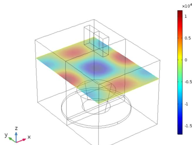
FIGURE 7 The snapshots of electric field distribution at middle layer in z direction of the microwave heating cavity with upper port position
