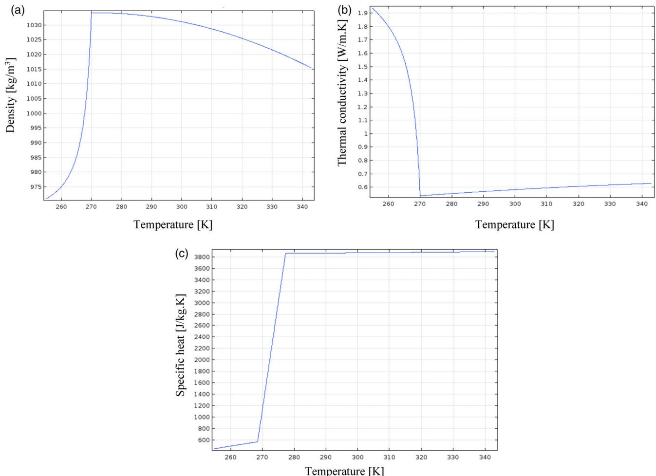
**FIGURE 2** Thermal properties of sample as a function of temperature from  $-18$  to  $80^{\circ}\text{C}$  (a) density, (b) thermal conductivity, and (c) specific heat
