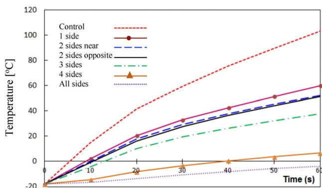
**FIGURE 6** The average calculated temperature inside the sample during microwave heating for 60 s at various resonator areas: case of side port
