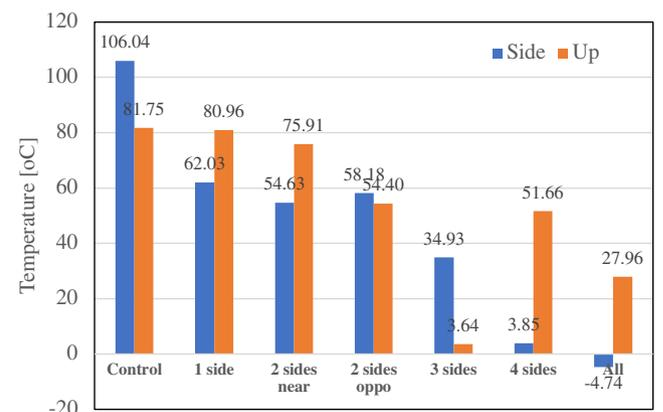
FIGURE 9 The average temperature comparison by waveguide position at various resonator areas after microwave heating process for 60 s
