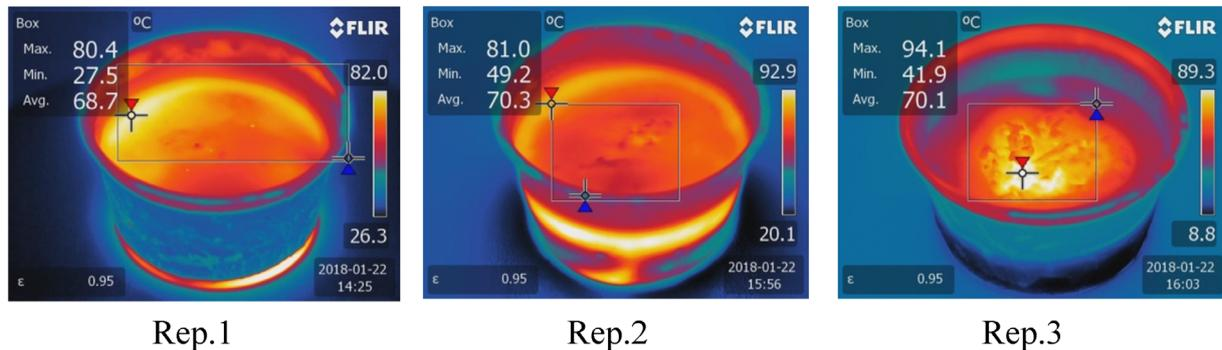
**FIGURE 4** Thermal image of frozen rice congee with package and resonator after subjected to microwave power 800 W, 2.45 GHz for 300 s
