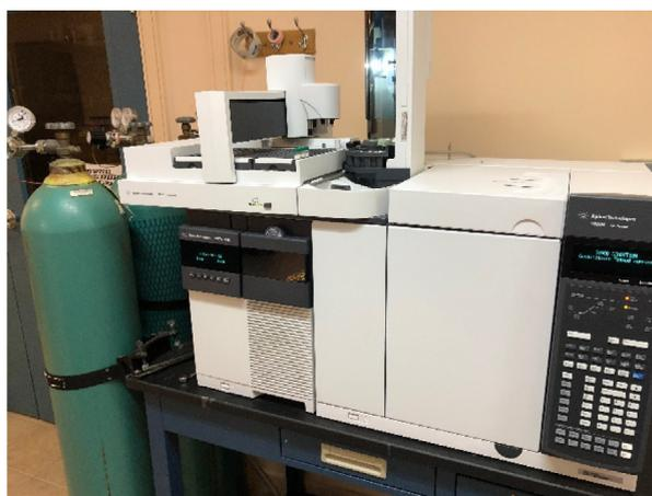
Fig. 1. GS-MS device (Agilent 5977B) used for analysing biofuel.
