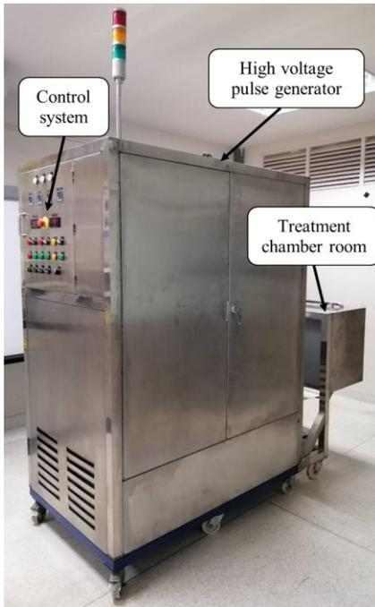
Fig. 4. The PEF system for CJ treatment.
