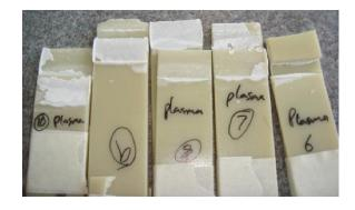
Zytel Lap Shear Failure Stress
