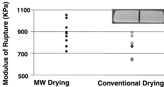
FIG. 6. Modulus of rupture (MOR) of tableware product.
