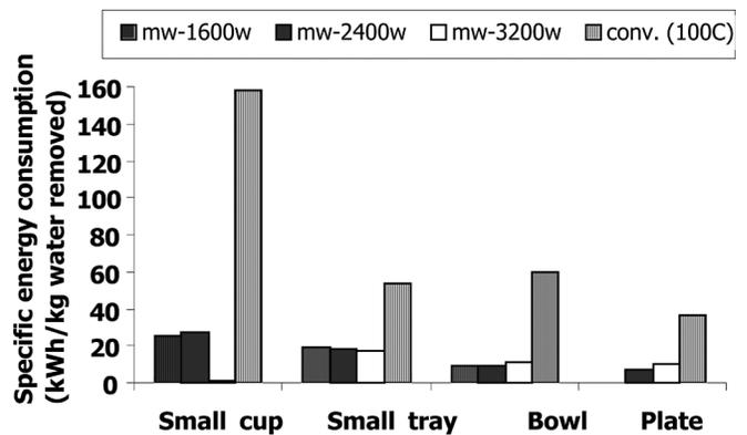
FIG. 3. Preliminary results of specific energy consumption.
