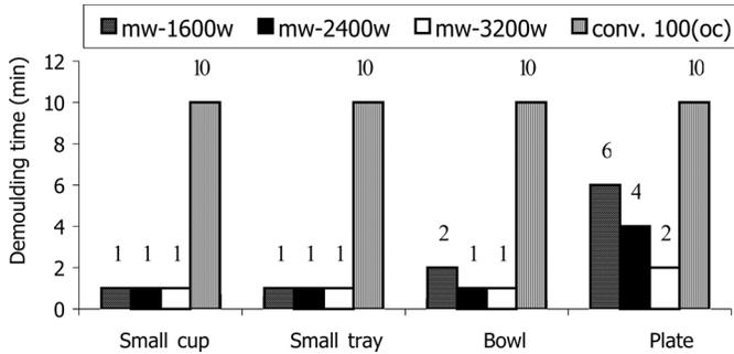
FIG. 4. Demolding time for tableware under conventional vs. microwave drying.
