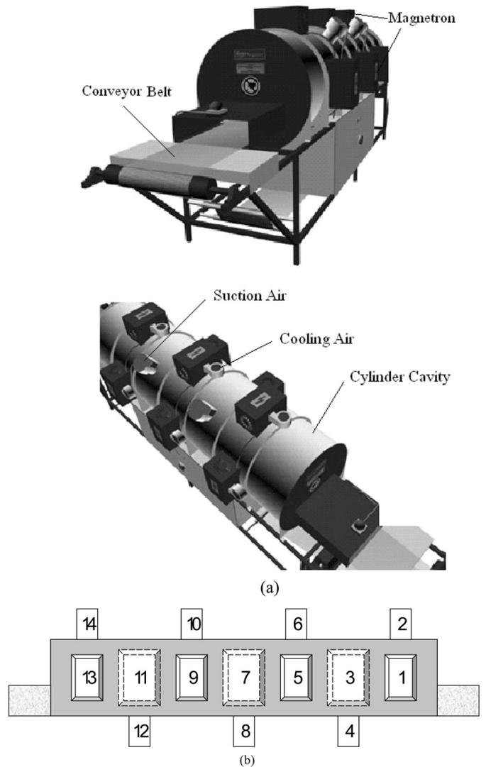
FIG. 1. (a) Microwave continuous belt dryer for drying tableware products, (b) location of 14 magnetrons.
