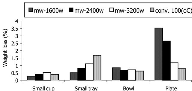
FIG. 5. Weight loss of various types of tableware under conventional vs. microwave drying.
