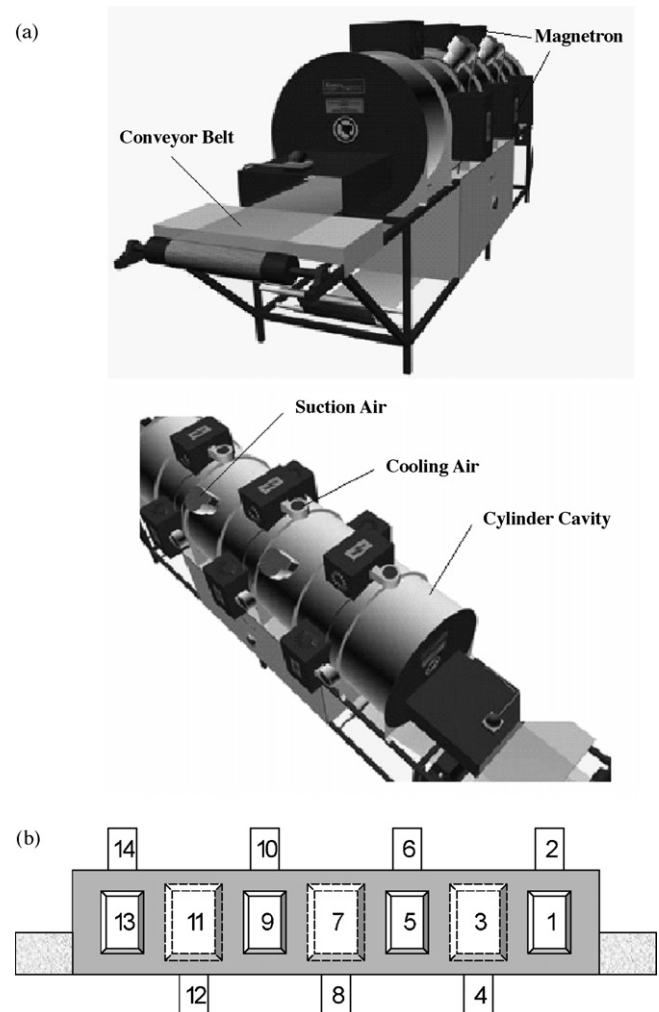
Fig. 1. (a) Continuous microwave belt drier for drying tableware product, (b) location of 14 magnetrons.
