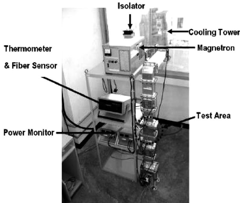
FIG. 1. Microwave using a rectangular waveguide.
