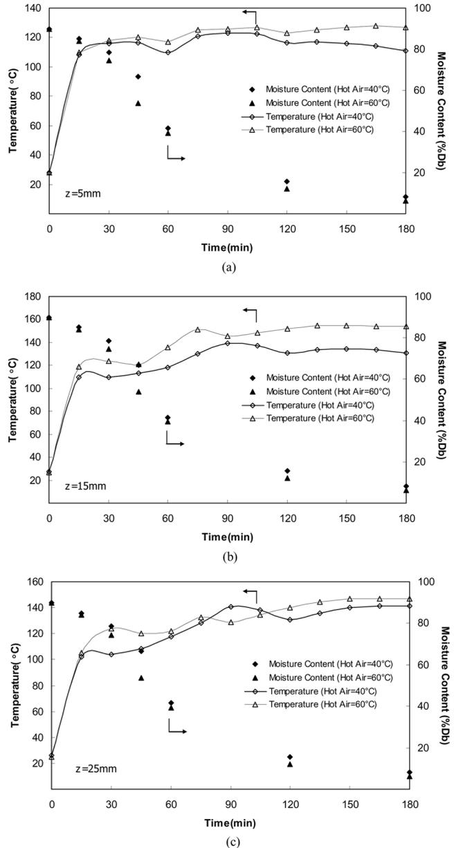
FIG. 8. Temperature and moisture profiles with respect to elapsed time;  $P = 100$  W, sample thickness of 50 mm:  $z = 5$  mm;  $z = 15$  mm; and  $z = 25$  mm.
