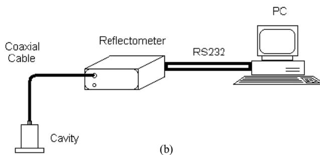
FIG. 4. Portable dielectric network analyzer.
