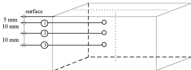
FIG. 3. Positions of temperature measurement.
