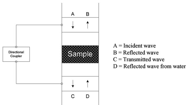
FIG. 2. Microwave power measurement.
