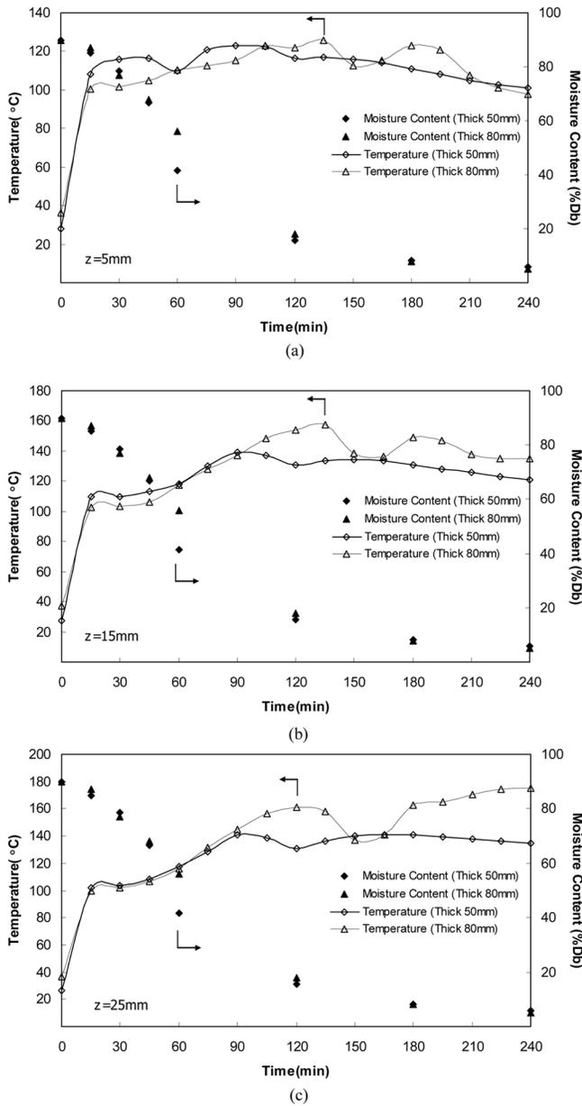
FIG. 11. Temperature and moisture profiles with respect to elapsed time;  $P = 100\text{ W}$ ,  $T_{\infty} = 40^{\circ}\text{C}$ : (a)  $z = 5\text{ mm}$ ; (b)  $z = 15\text{ mm}$ ; and (c)  $z = 25\text{ mm}$ .
