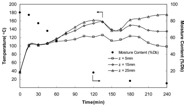
FIG. 13. Temperature and moisture profiles with respect to elapsed time;  $P = 100$  W, sample thickness of 80 mm,  $T_\infty = 40^\circ\text{C}$ .
