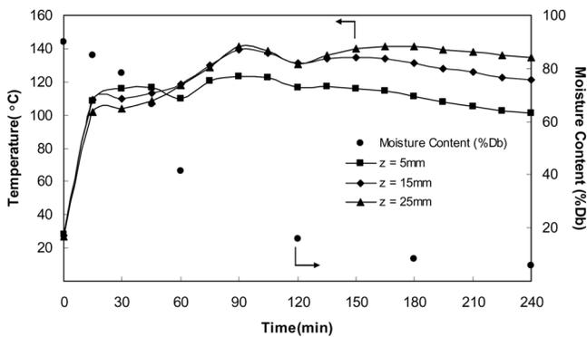
FIG. 7. Temperature and moisture profiles with respect to elapsed time;  $T_{\infty} = 40^{\circ}\text{C}$ , sample thickness of 50 mm,  $P = 100$  W.
