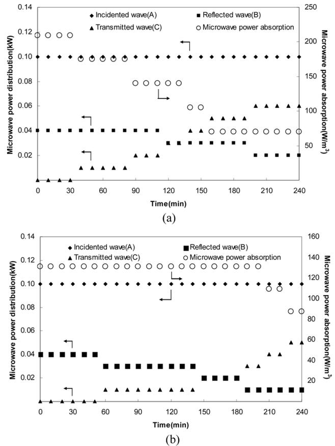
FIG. 12. Microwave power distribution and microwave power absorption with respect to elapsed time;  $P = 100\text{ W}$ ,  $T_{\infty} = 40^{\circ}\text{C}$ : (a) sample thickness of  $50\text{ mm}$  and (b) sample thickness of  $80\text{ mm}$ .
