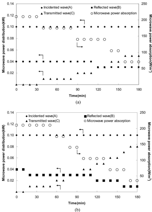
FIG. 9. Microwave power distribution and microwave power absorption with respect to elapsed time;  $P = 100\text{ W}$ , Sample thickness of  $50\text{ mm}$ : (a)  $T_{\infty} = 40^{\circ}\text{C}$  and (b)  $T_{\infty} = 60^{\circ}\text{C}$ .
