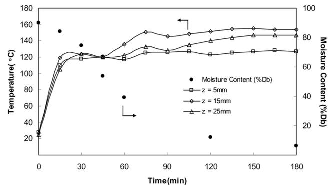
FIG. 10. Temperature and moisture profiles with respect to elapsed time;  $P = 100\text{ W}$ , sample thickness of  $50\text{ mm}$ ,  $T_{\infty} = 60^{\circ}\text{C}$ .
