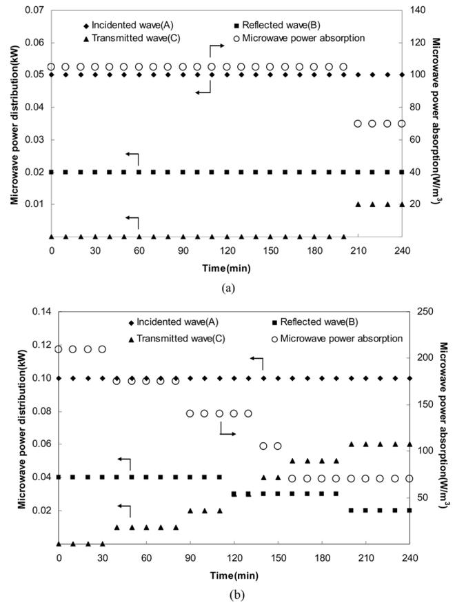
FIG. 6. Microwave power distribution and microwave power absorption with respect to elapsed time;  $T_{\infty} = 40^{\circ}\text{C}$ , sample thickness of  $50\text{ mm}$ :  $P = 50\text{ W}$ ;  $P = 100\text{ W}$ .
