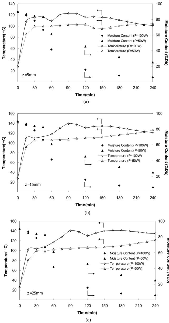
FIG. 5. Temperature and moisture profiles with respect to elapsed time;  $T_{\infty} = 40^{\circ}\text{C}$ , sample thickness of  $50\text{ mm}$ : (a)  $z = 5\text{ mm}$ ; (b)  $z = 15\text{ mm}$ ; and (c)  $z = 25\text{ mm}$ .
