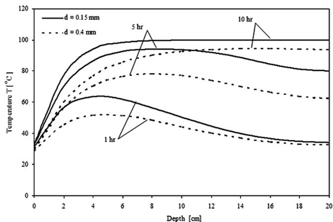
FIG. 13. Temperature profiles at various particle sizes ( $f = 2.45$  GHz,  $E_{in} = 4,200$  V/m,  $S_{in} = 0.7$ ).
