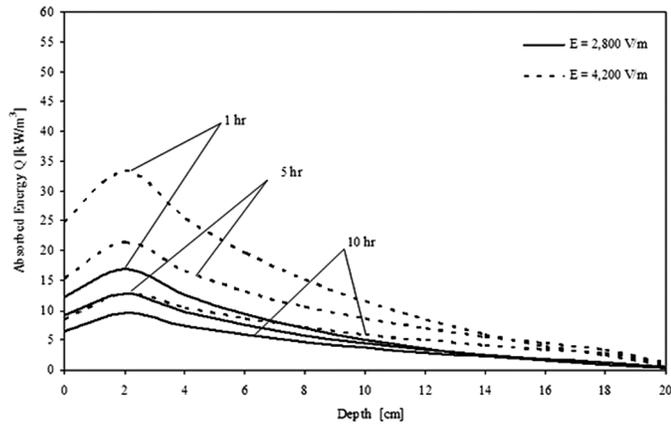
FIG. 19. Energy-absorbed profiles at various electric field intensities ( $f=2.45$  GHz,  $d=0.15$  mm,  $S_{in}=0.7$ ).
