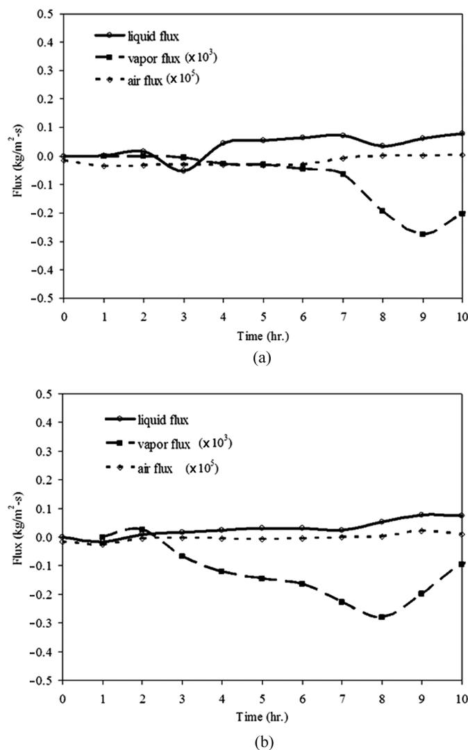
FIG. 11. Flux profiles at 4 cm in case of frequency (a) 2.45 GHz and (b) 5 GHz ( $d=0.15$  mm,  $E_{in}=4,200$  V/m,  $S_{in}=0.7$ ).
