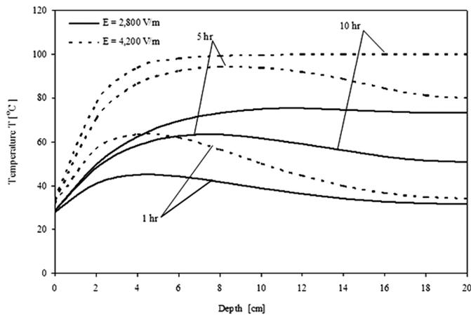
FIG. 20. Temperature profiles at various electric field intensities ( $f=2.45$  GHz,  $d=0.15$  mm,  $S_{in}=0.7$ ).
