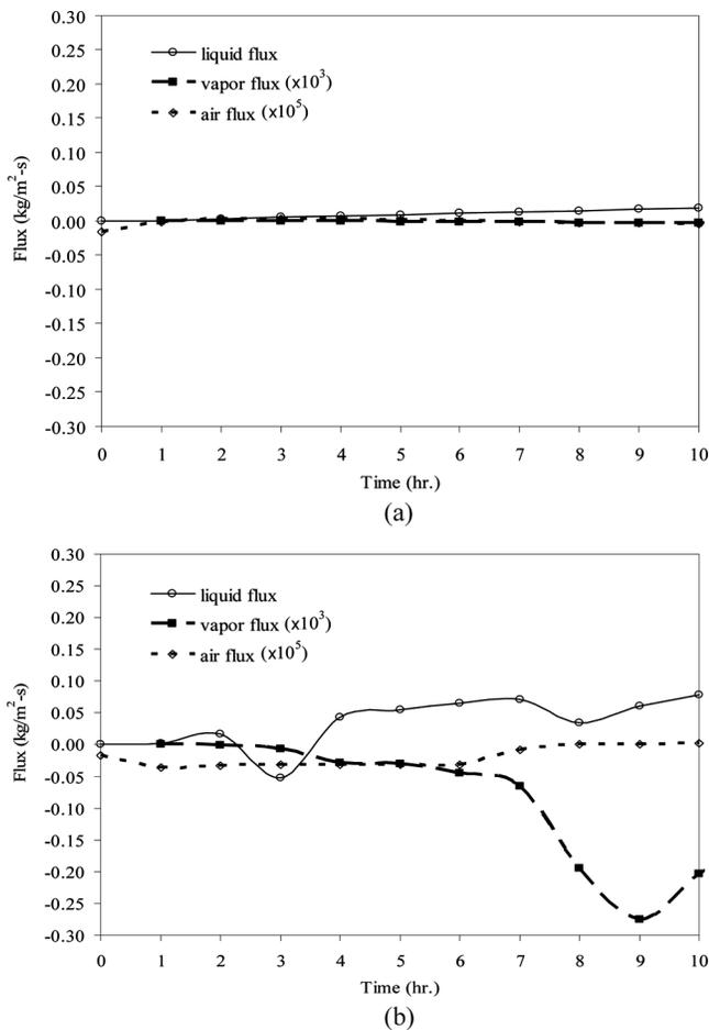
FIG. 25. Flux profiles at 4 cm in case of electric field intensity (a) 2,800 V/m and (b) 4,200 V/m ( $f = 2.45$  GHz,  $d = 0.15$  mm,  $S_m = 0.7$ ).
