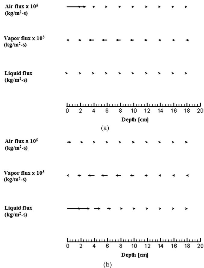
FIG. 10. Fluid movement pattern at 10h in case of frequency (a) 2.45 GHz (vector length [relative]: 1 grid units/magnitude) and (b) 5 GHz (vector length [relative]: 12 grid units/magnitude).
