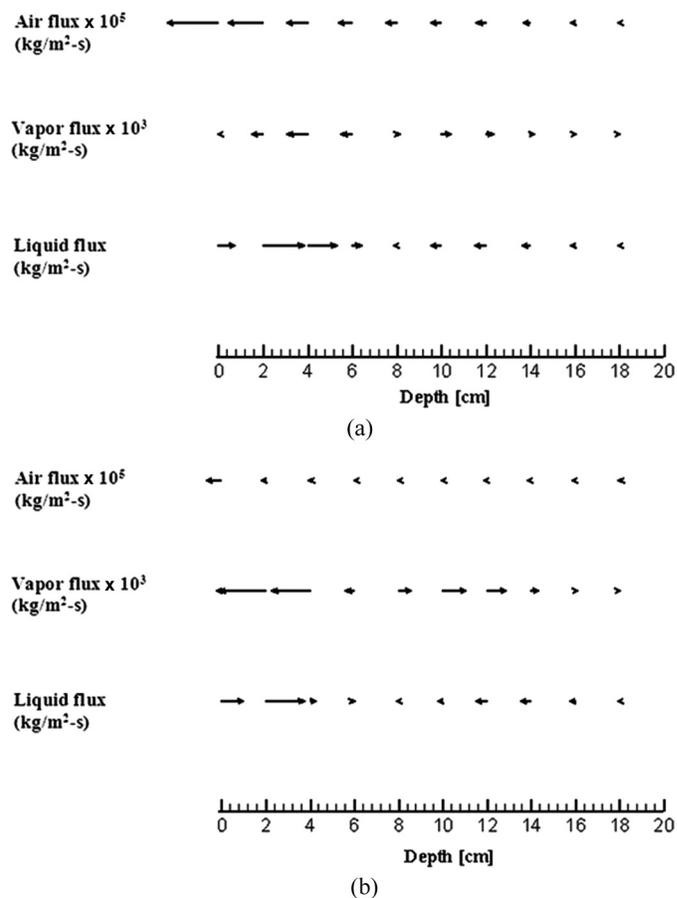
FIG. 9. Fluid movement pattern at 4 h in case of frequency (a) 2.45 GHz (vector length [relative]: 30 grid units/magnitude) and (b) 5 GHz (vector length [relative]: 10 grid units/magnitude).
