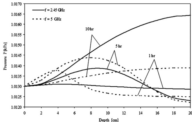
FIG. 8. Pressure distribution at various frequencies ( $d=0.15$  mm,  $E_{in}=4,200$  V/m,  $S_{in}=0.7$ ).
