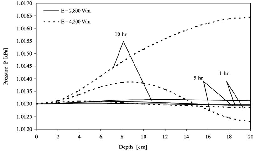
FIG. 22. Pressure distribution at various electric field intensities ( $f=2.45$  GHz,  $d=0.15$  mm,  $S_{in}=0.7$ ).
