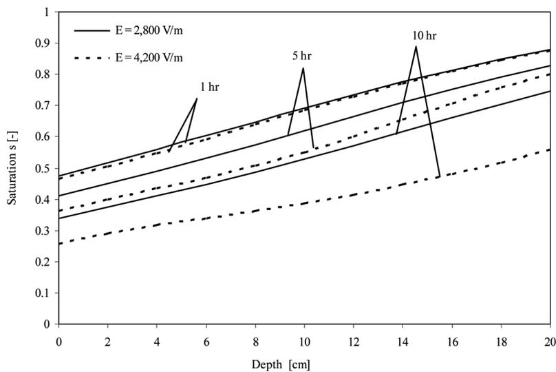
FIG. 21. Moisture profiles at various electric field intensities ( $f=2.45$  GHz,  $d=0.15$  mm,  $S_{in}=0.7$ ).
