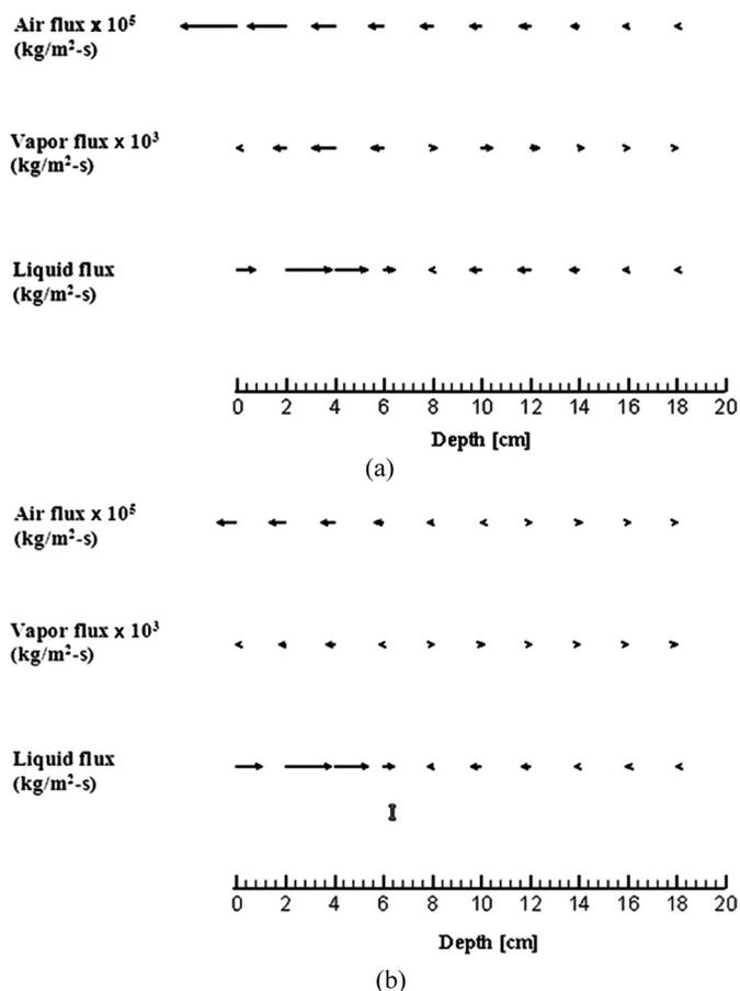
FIG. 16. Fluid movement pattern at 4h in case of particle size (a) 0.15 mm (vector length [relative]: 30 grid units/magnitude) and (b) 0.4mm (vector length [relative]: 65 grid units/magnitude).
