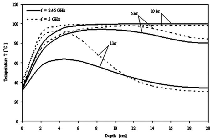
FIG. 6. Temperature profiles at various frequencies ( $d=0.15$  mm,  $E_{in}=4,200$  V/m,  $S_{in}=0.7$ ).
