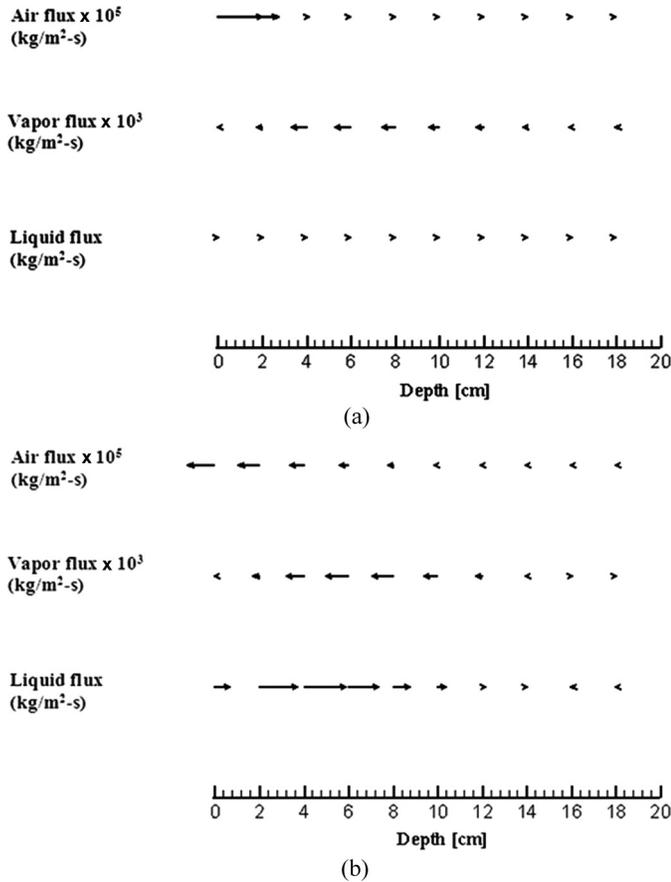
FIG. 17. Fluid movement pattern at 10h in case of particle size (a) 0.15 mm (vector length [relative]: 1 grid units/magnitude) and (b) 0.4 mm (vector length [relative]: 35 grid units/magnitude).
