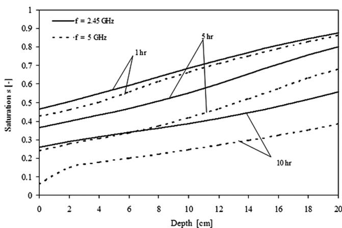
FIG. 7. Moisture profiles at various frequencies ( $d=0.15$  mm,  $E_{in}=4,200$  V/m,  $S_{in}=0.7$ ).
