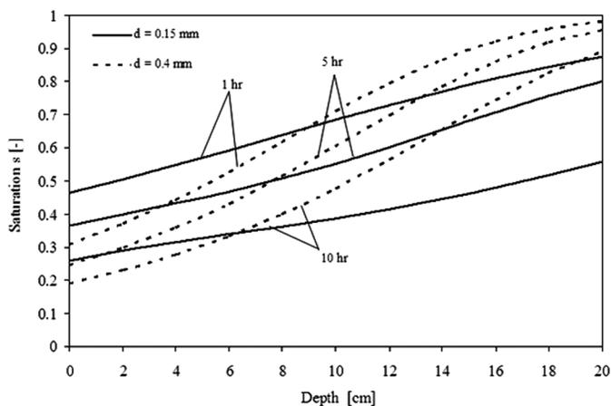
FIG. 14. Moisture profiles at various particle sizes ( $f = 2.45$  GHz,  $E_{in} = 4,200$  V/m,  $S_{in} = 0.7$ ).
