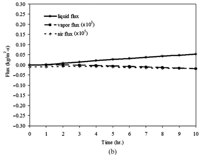
FIG. 18. Flux profiles at 4 cm in case of particle size (a) 0.15 mm and (b) 0.4 mm ( $f=2.45$  GHz,  $E_{in}=4,200$  V/m,  $S_{in}=0.7$ ).
