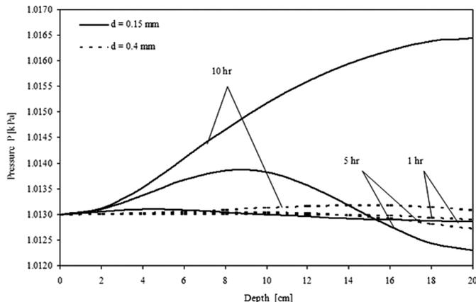
FIG. 15. Pressure distribution at various particle sizes ( $f = 2.45$  GHz,  $E_{in} = 4,200$  V/m,  $S_{in} = 0.7$ ).
