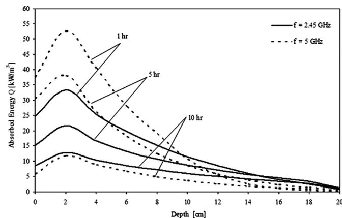
FIG. 5. Energy absorbed profiles at various frequencies ( $d = 0.15$  mm,  $E_{in} = 4,200$  V/m,  $S_{in} = 0.7$ ).
