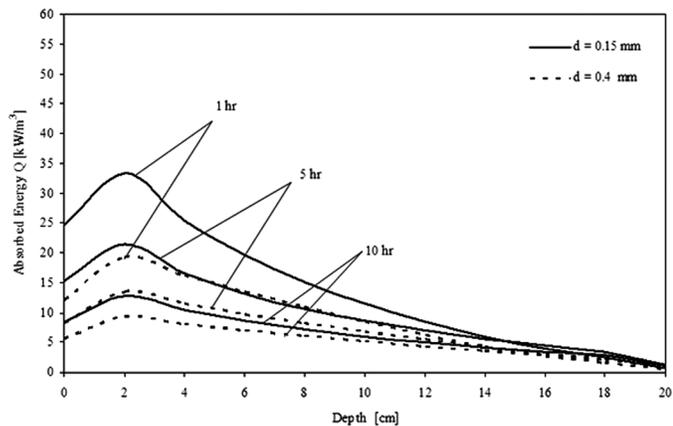
FIG. 12. Energy-absorbed profiles at various particle sizes ( $f = 2.45$  GHz,  $E_{in} = 4,200$  V/m,  $S_{in} = 0.7$ ).
