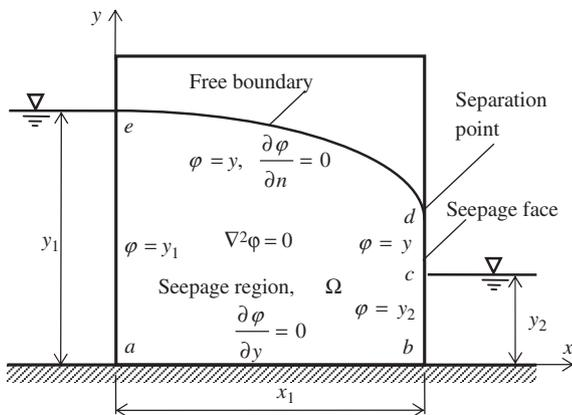
Fig. 1. Flow through a 2D rectangular dam.
