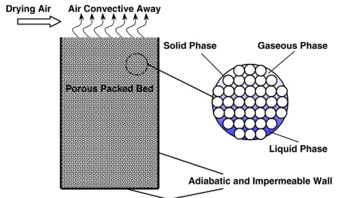
Fig. 3. Configuration of porous packed bed.
