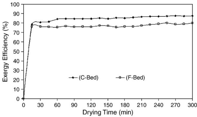
Fig. 9. Variation of exergy efficiency with different packed bed.
