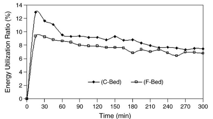
Fig. 8. Variation of energy utilization ratio with different packed bed.
