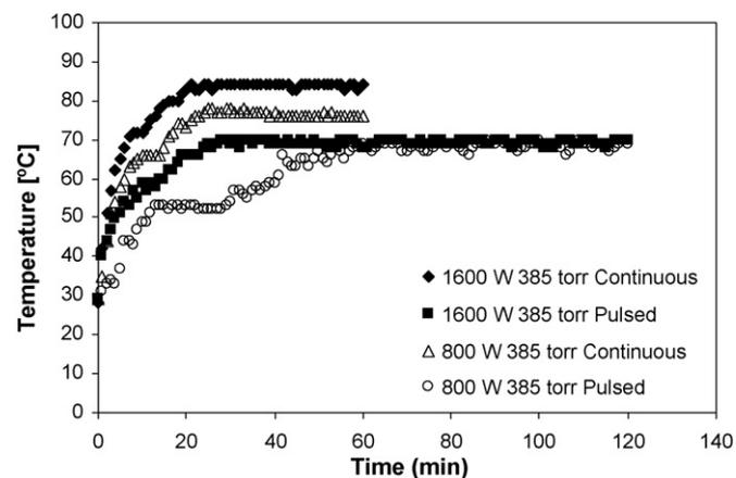
Fig. 7. Variations of cavity temperature with drying time using continuous microwave operating mode and pulsed microwave operating mode at 385 Torr vacuum pressure.
