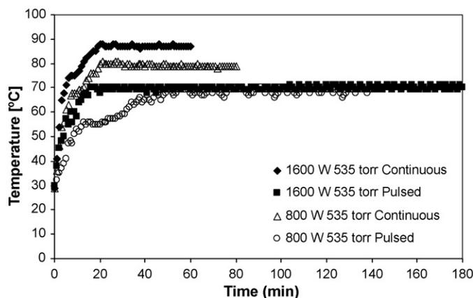
Fig. 8. Variations of cavity temperature with drying time using continuous microwave operating mode and pulsed microwave operating mode at 535 Torr vacuum pressure.
