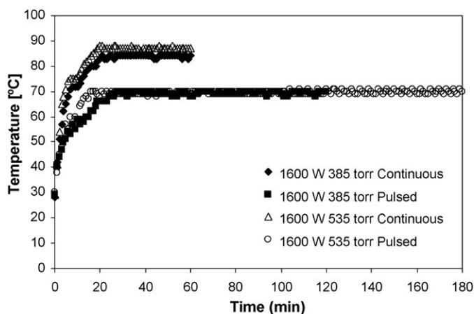
Fig. 5. Variations of cavity temperature with drying time using continuous microwave operating mode and pulsed microwave operating mode at 1600 W magnetron power.
