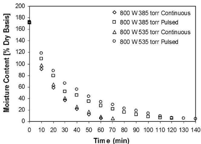
Fig. 4. Variations of moisture content with drying time using continuous microwave operating mode and pulsed microwave operating mode at 800 W magnetron power.
