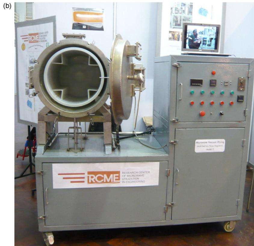
**Fig. 2.** The commercialized biomaterials drier. (a) Detail of the system. (b) MW drying experiments were carried out at the Research Center of Microwave Utilization in Engineering (R.C.M.E.) Department of Mechanical Engineering, Faculty of Engineering, Thammasat University.
