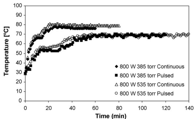
Fig. 6. Variations of cavity temperature with drying time using continuous microwave operating mode and pulsed microwave operating mode at 800 W magnetron power.
