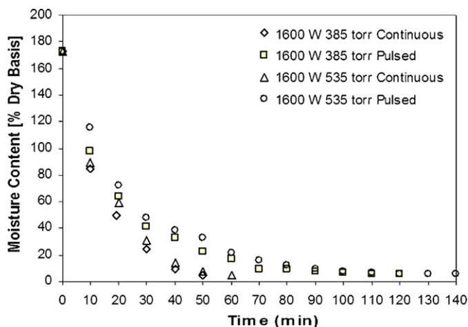
Fig. 3. Variations of moisture content with drying time using continuous microwave operating mode and pulsed microwave operating mode at 1600 W magnetron power.
