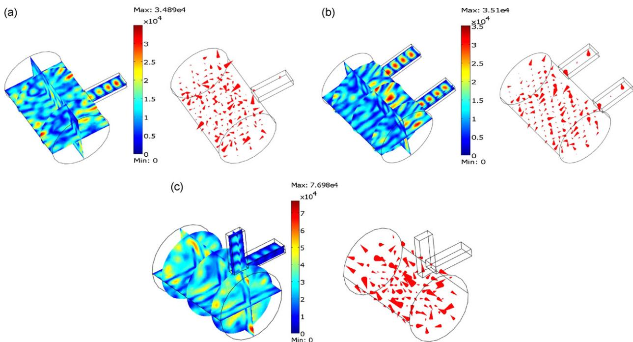
**Fig. 1.** The simulation of electric field distribution (V/m) in multimode cavity (Slice Plot Type and Arrow Plot Type). (a) Simulated electric field distribution and arrow plot in multimode cavity with one-feed single magnetron. (b) Simulated electric field distribution and arrow plot in multimode cavity with symmetrical double-feed two magnetrons. (c) Simulated electric field distribution and arrow plot in multimode cavity with unsymmetrical double-feed two magnetrons.
